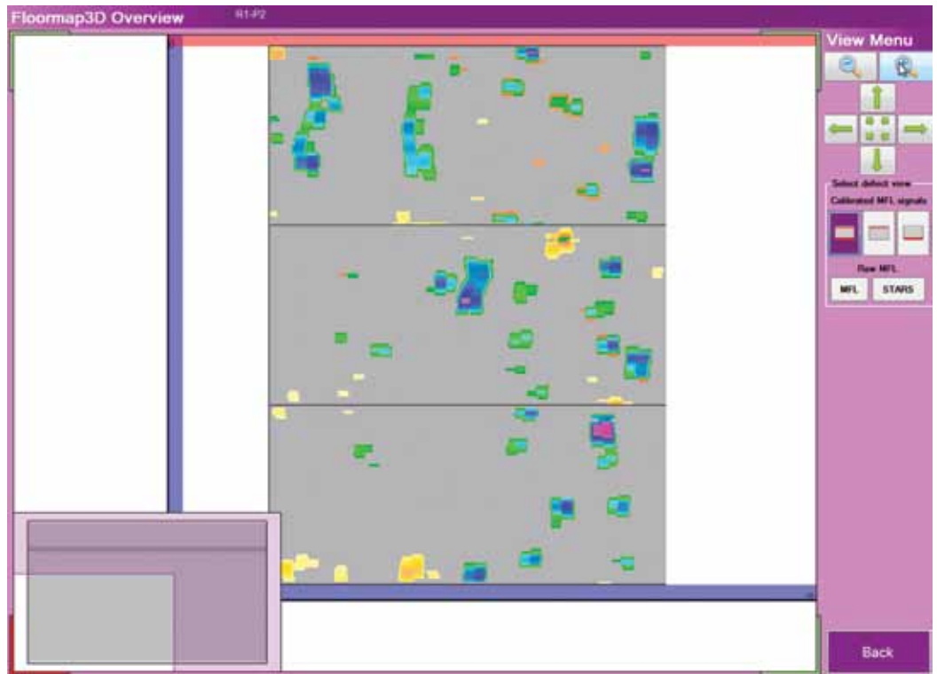
Sample data report from Silverwing Floormap3D showing defect indications on the tank floor
